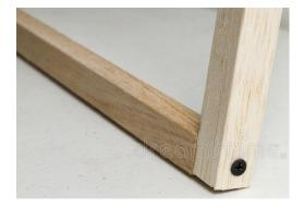
(20mm) higher and lower than the picture so they can connect to the top and bottom beams. For a diagonalcorner frame, all beams must be 4cm (40mm) longer than the picture at **every corner**, so they can be glued to the neighboring beams.
